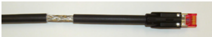
Fig. 10-20: Foil shield removed
