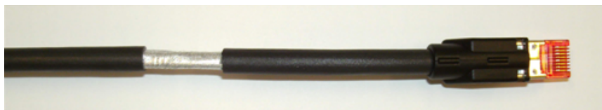
Fig. 10-18: CDI cable with partially removed jacket
