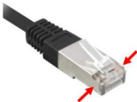
Fig. 10-16: RJ45 plug shielding areas
