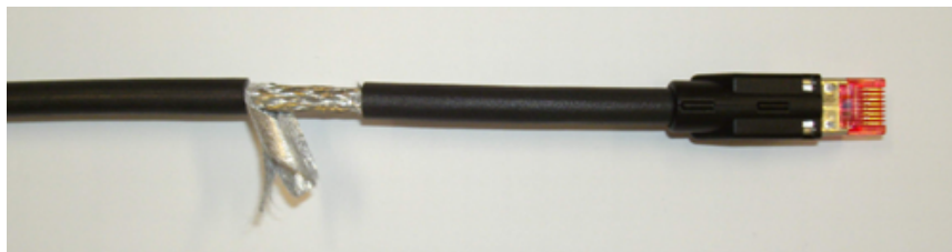
Fig. 10-19: Foil shield of the CDI cable
