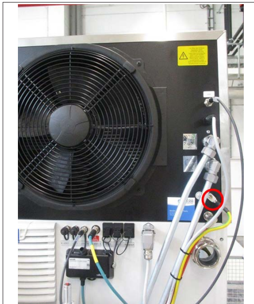
Fig. 22: Connecting the protective grounding conductor
