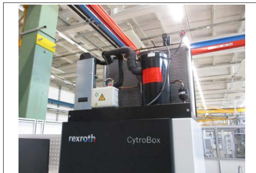
Fig. 15: Aligning the compressor cooler
