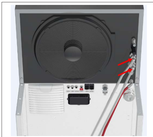
Fig. 18: Connecting the hydraulic lines
