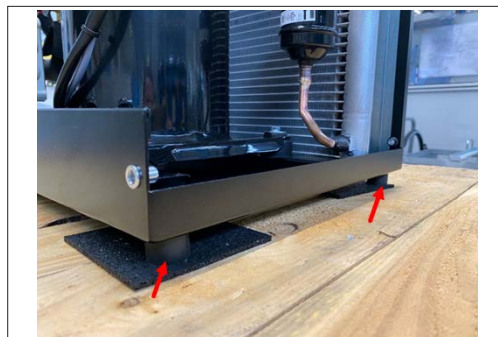
Fig. 12: Removing the rubber feet
