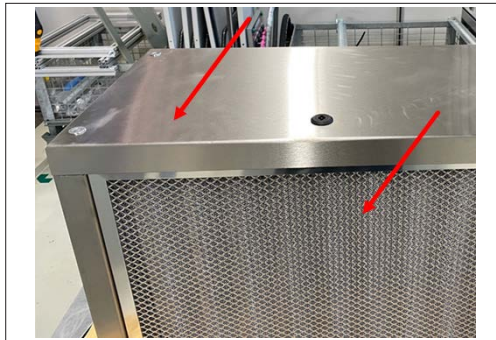
Fig. 17: Attaching the filter element mat and housing
